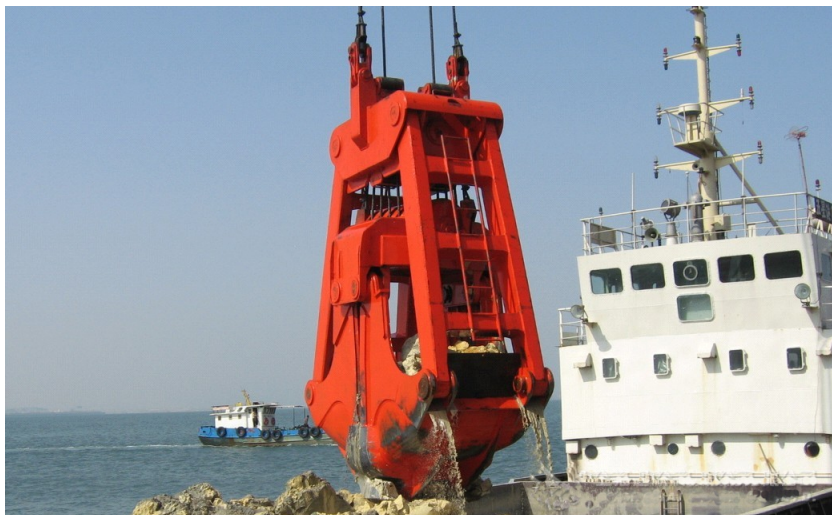
Underwater Dredging Grab Working picture
