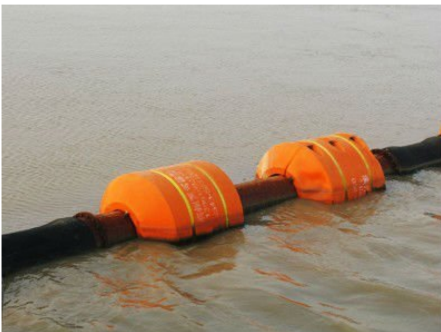
dredging floater with pipe
