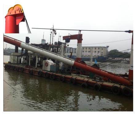
The dredge anchor boom'length depends on the stability and the dimensions of the pontoon. It can determines how far the anchor can be placed outside the Cutter Suction Dredger.
