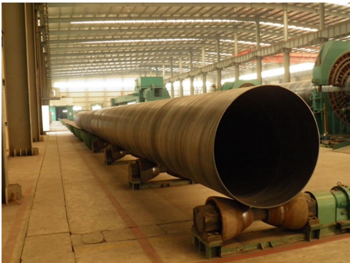
SSAW Dredging Steel Pipe in Workshop
